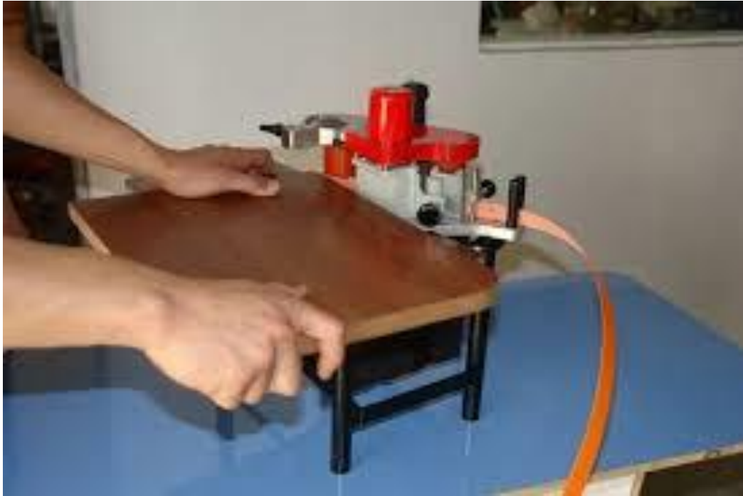
Image: Application of PVC edge banding in furniture manufacturing
