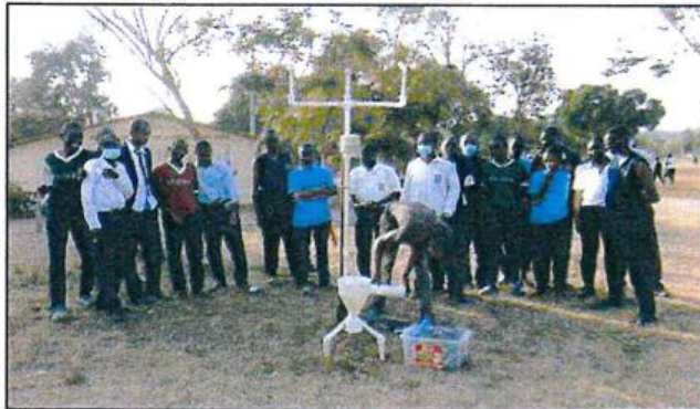
KSA technical staff carrying out maintenance of 3D-PAWS (3-D Printed Automatic Weather Stations) in schools.
