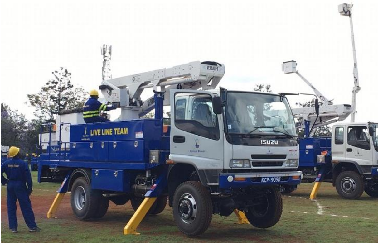
Live line maintenance trucks used by Kenya Power & Lighting Company to ensure continuity of power supply during maintenance
